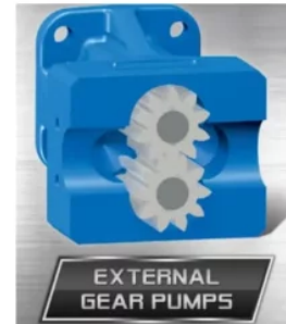
Flow path through an external Gear Pump
